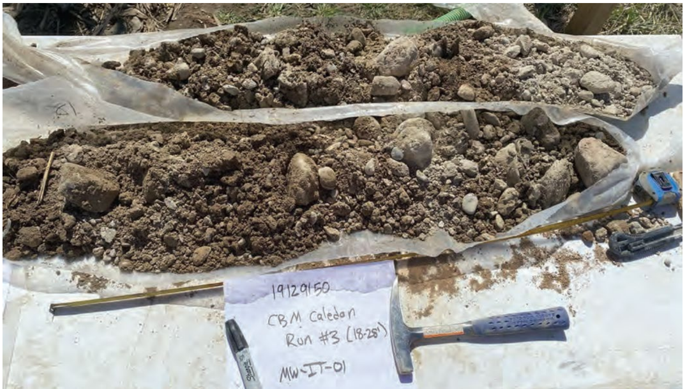
Figure 4: Continuous Core at MW-IT-01 within Proposed Infiltration Trench Zone 2
