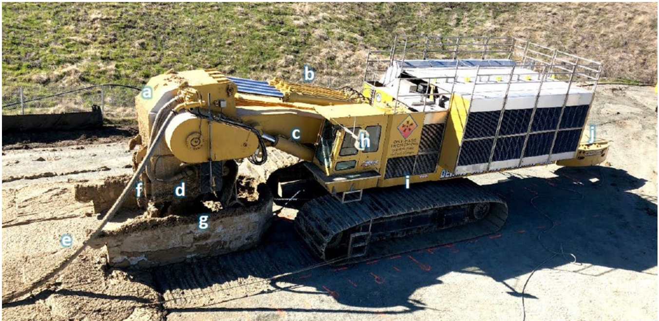
Figure 17: One-Pass Trenching Method a) Digging box. b) Stick (pivot) cylinders. c) Lift (stroke) cylinders. d) Boom. e) Water supply line. f) Digging/mixing chain. g) Drag Box. h) Cab. i) Tracks. j) Counterweight (DeWind, 2025).
