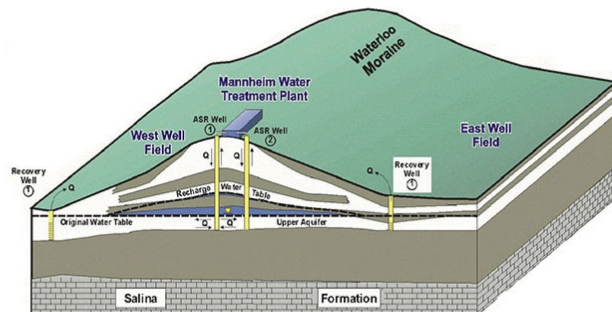
Figure 5: Mannheim Aquifer Storage and Recovery System Conceptual Configuration (Camilleri, 2019)
